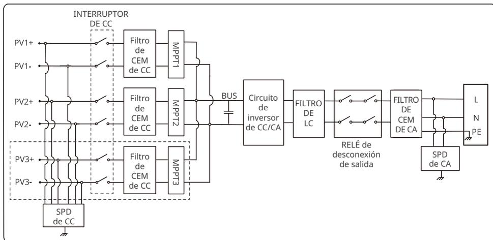
PV3+/PV3- solo para GW5000-MS-30, GW6000-MS-30, GW7000-MS-30, GW8500-MS-30 y GW10K-MS-30.
